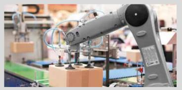
Determining the position of a package so that it can be gripped by a robotic arm
