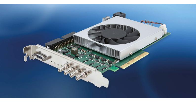
The new four-channel image acquisition card captures image data from the camera at up to 50 Gbps and can be used in multi-camera and multi-board systems for real-time applications with the lowest latencies. The frame grabber is characterized by high speed as well as extensive image pre-processing and trigger functions (connection of an additional TTL trigger board). It is suitable for all common CXP-12 cameras (CoaXPress 2.0) and CXP-6 cameras (CoaXPress 1.1.1).
