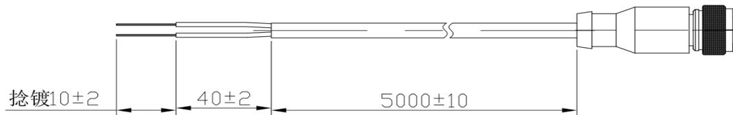
Ethernet: Type A code M12 male terminal to RJ45 (UTP-CAT5E network cable)
