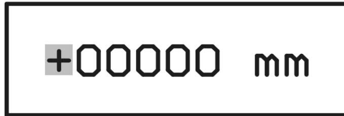
Meaning of offset: measured distance +set offset=displayed and output distance;
