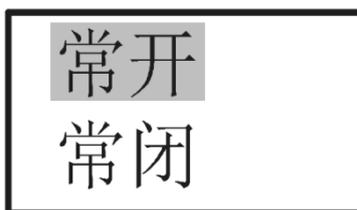
After entering the output status menu bar, the highlighted part is the current output status. Press Page Up/Page Down to switch the output state, and press “Set” to set the output state. After setting it will automatically return to the setting menu page.
