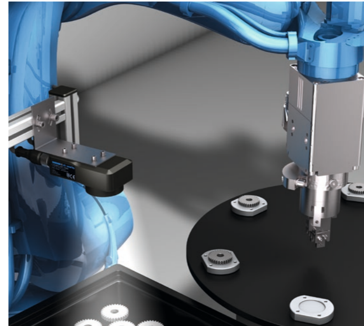
Inspection of parts and robotic pick & place
