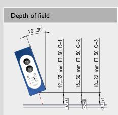
The depth of field of the FT 50 C also varies depending on the light spot geometry:
