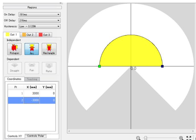
Figure 4.2.1.2.3.1-2 Example of arc configuration by numerical input
