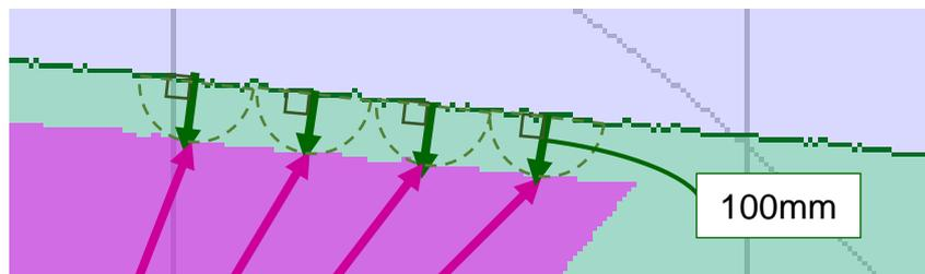
Figure 4.2.1.2.4-7 Distance offset using the Erosion method
