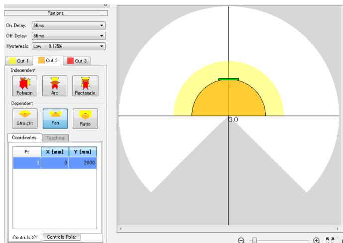
Figure 4.2.1.2.3.2-2 Example of fan shape by numerical input
