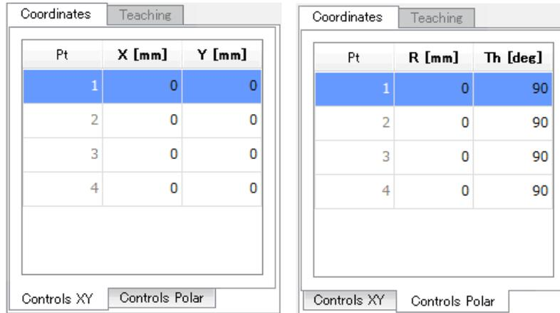
Figure 4.2.1.2.3.1-1 Example of default state of Numerical input screen during independent rectangle selection (Left: XY Coordinates, Right: Polar Coordinates)
