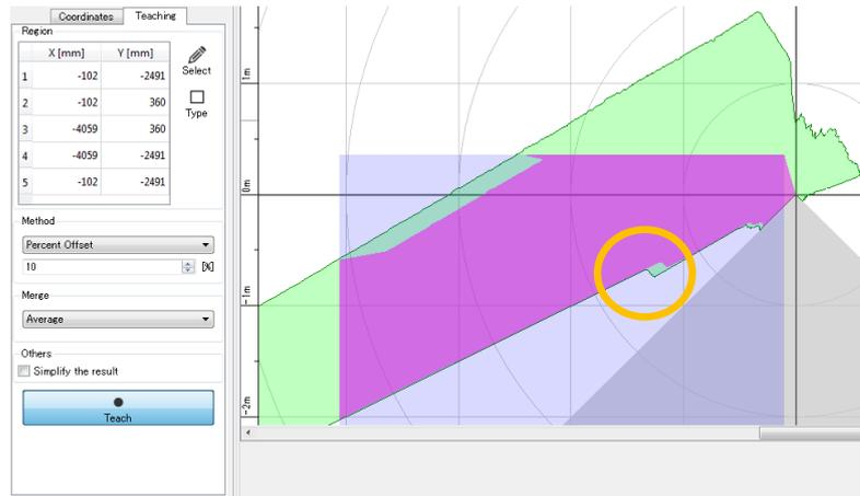
Figure 4.2.1.2.4-11 Distance offset using the Percent Offset method
