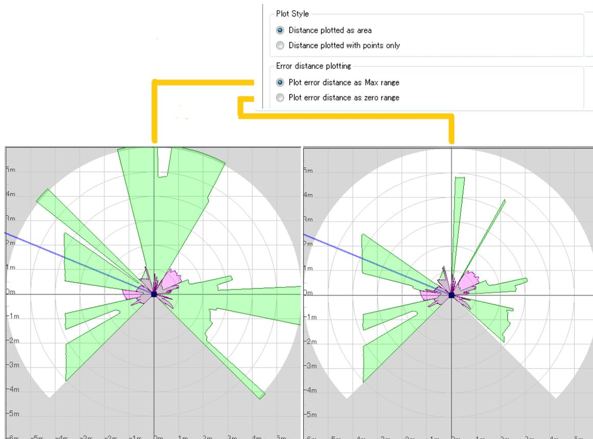
Figure 4.4-6 Changing the display of the output data (top), changing the display of the error data (bottom)
