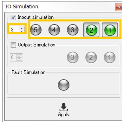
Figure 4.6-3 Input simulation numerical input and lamps
