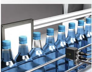
Fill level checking and cover fit
