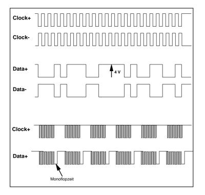
The clock pulses and data are differentially transmitted by means of cable transmitters with TTL levels and received by means of optocouplers to protect them from damage resulting from interference, potential differences, or polarity reversal.
