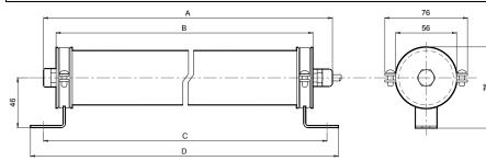
Cable lenght: 10m Cables of different lengths available on request. Ø max (mm) = 5,8
