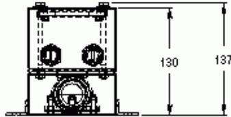
Enclosure is constructed of 16 gauge 316 stainless steel.
