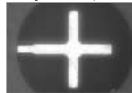
BGA Alignment Mark Inspection
