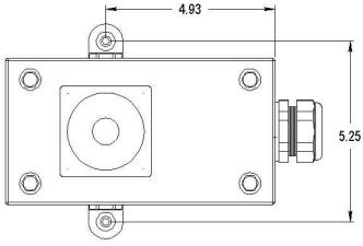
Max camera lens height: 2.98" for standard enclosure Extended enclosure available for long lenses
