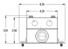
Enclosure is constructed of 18 gauge Type 316 stainless steel.
