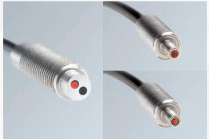
Fibre optic transmitters and receivers run in two separate sheaths, which are connected to the sensor's appropriate optical components by means of the glass fibre coupling. With conventional fibre optics (left-hand picture), both fibres run parallel to one another whilst with co-axial fibre optics the fibre-optic receivers run co-axially around the transmitter fibres. This is of advantage when using an additional optic, e.g. a smaller light spot and a better small part detection.
