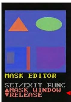
Press [SET] four times to switch to the mask adding/releasing function applying to square in mask window.
