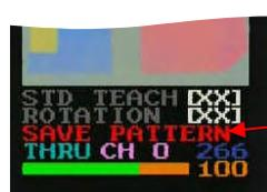
During the writing process, the characters **SAVE PATTERN** is displayed red. When this turns to yellow, the process is completed.
