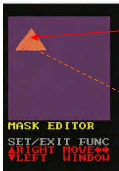
Moving the mask window to the red triangle, makes the display only with the red color, and all the other part will be displayed purple.
