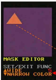
To solve the problem, press [SET] three times to make the display like this. This is the function to adjust the selected color width.
