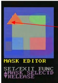
In this example, press **[DOWN]** to clear the masking under the red triangle .
