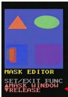
Press [SET] four times to switch to the function to add/clear the mask to the square part of mask window.
