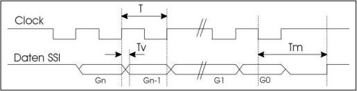
T = Duration of clock signal, minimum 2  $\mu$ Sec = 500 kHz, max. 13  $\mu$ Sec = 77kHz Tv = Delay time max. 360 ns
