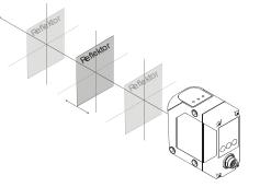
Different reflector types are available according to the distance range required. Only use the reflectors specified below.
