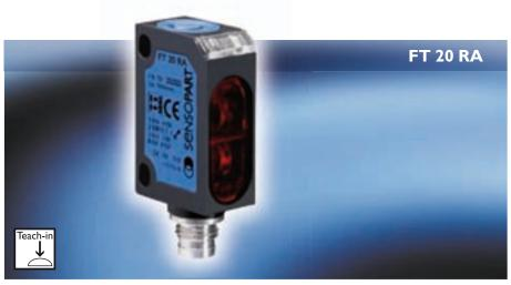
The FT 20 RA has a signal output in addition to the analogue voltage output and offers the possibility of defining a screening function using two switch points. It can thus be used as a threshold switch.
