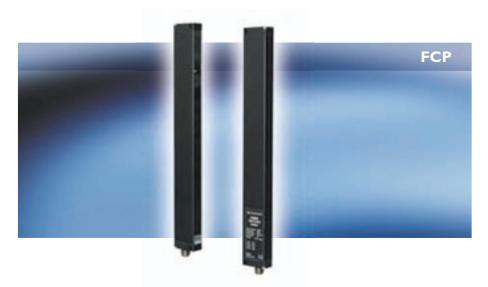
The FCP light grid measures the height of an object in the measuring field and is thus suitable for detecting, measuring and counting objects of different shapes and sizes. The devices in this series are available with measuring field heights of 100, 150 or 300 mm with resolutions from 5 mm upwards.
