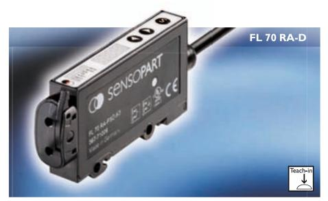
The FL 70 RA-D is a high-end fibre-optic amplifier with a 4 digit display. This version has an analogue and signal output and supplies a signal which is proportional to the reflectivity of the detected object and which in turn is proportional to the distance, cross-section, etc., when reflectivity from the object is constant.
