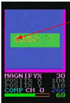
Even though the magnification compensation is activated, the magnifying rate varies depending on the pixel number, to cause much error. When the pixels of detection target color varies, the magnification compensation is not recommended.
