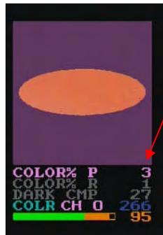
Increase the COLOR % P (color margin for position compensation) of the setting value to completely cover the colors to be selected.
