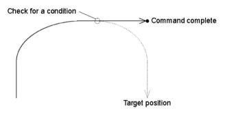
Command No. 952 can then be used to verify whether the Sense condition was satisfied and the manipulator stopped prior to its target position or that the Sense condition was not satisfied and the manipulator continued until stopping at its target position.
