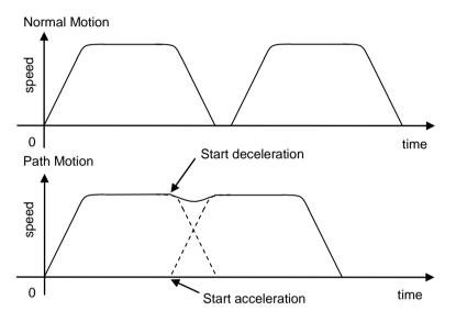
When CP is On, path motion will continue without full deceleration between two CP motion (Arc, Arc3, Jump3, Jump3CP, Move), or two PTP motion (Go, Jump). In contrast, full deceleration will occur between a CP motion and a PTP motion.
