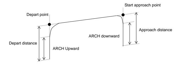
Jump3CP uses the SpeedS speed value and AccelS acceleration and deceleration values. Refer to *Using Jump3CP with CP* below on the relation between the speed/acceleration and the acceleration/deceleration. If, however, the ROT modifier parameter is used, Jump3CP uses the SpeedR speed value and AccelR acceleration and deceleration values. In this case SpeedS speed value and AccelS acceleration and deceleration value have no effect.
