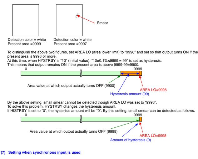
When imaging by the synchronous input, sometimes, you may want to turn ON the output only when a work is OK.
