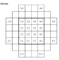
Points that represent divisions of a pallet are automatically assigned division numbers, which, in this example, begin at P1. These division numbers are also required by the Pallet Function.
