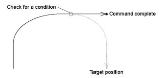
The JS or Stat commands can then be used to verify whether the Sense condition was satisfied and the robot stopped prior to its target position or that the Sense condition was not satisfied and the robot continued until stopping at its target position.
