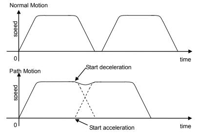
When CP is On, path motion will continue without full deceleration between two CP motions (Arc, Arc3, Jump3, Jump3CP, Move), or two PTP motions (Go, Jump). In contrast, full deceleration will occur between a CP motion and a PTP motion.
