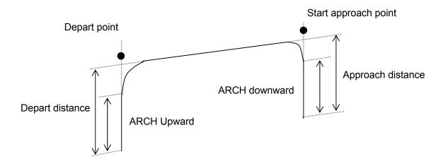
**Jump3CP** uses the SpeedS speed value and AccelS acceleration and deceleration values. Refer to *Using Jump3CP with CP* below on the relation between the speed/acceleration and the acceleration/deceleration. If, however, the ROT modifier parameter is used, **Jump3CP** uses the SpeedR speed value and AccelR acceleration and deceleration values. In this case SpeedS speed value and AccelS acceleration and deceleration value have no effect.
