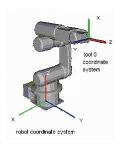
Tool 0 coordinate systems are defined for ceiling and wall mounted robots as shown in the figures below.
