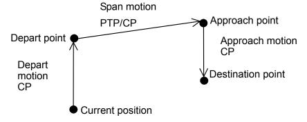
Arch motion is achieved by specifying the arch number. The arch motion for Jump3, Jump3CP is as shown in the figure below. For arch motion to occur, the Depart distance must be greater than the arch upward distance and the Approach distance must be greater than the arch downward distance.
