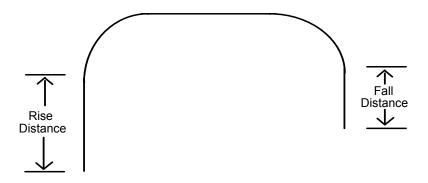
There are a total of 8 entries in the **Arch** Definition Table with 7 of them (0-6) being user definable. The 8th entry (**Arch** 7) is the default Arch which actually specifies no arch at all which is referred to as Gate Motion. (See Gate Motion diagram below) The Jump instruction used with the default **Arch** entry (Entry 8) causes the arm to do the following:
