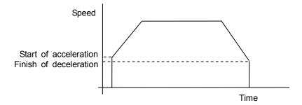
If omitted the finishing speed of deceleration, the speed set value is used.
