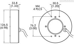
Click for Installation Models & Drawings ♦ UV LEDs have a considerably shorter half-life than other LEDs (<1000hrs). For this reason Ai recommends these LEDs be used in strobe mode only. applications requiring continuous 24v power, contact Ai for assistance.
