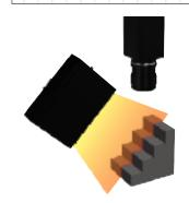
Molded pieces and other three-dimensional objects can also be inspected using line light.
