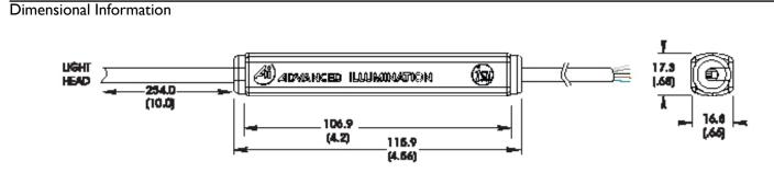
*The iSU is not detachable.* Standard location is 10" from the light head; if necessary, a different cable length and / or iSU location can be specified when ordering. Standard Cable Length (including ISU) is 1.5M (59").
