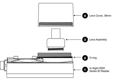
Figure 4: Lens Cover Installation/Removal
