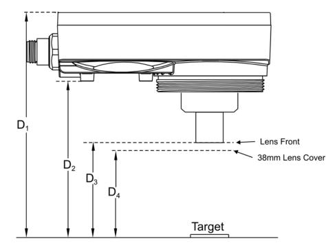
**Figure 5: Working Distance Dimensions**
