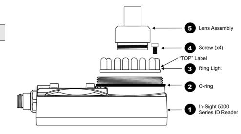
Figure 3: Ring Light Installation/Removal
