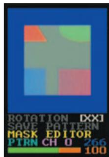
The masking window blinks. The status of the color detection window of the applied function used last time is reflected.
