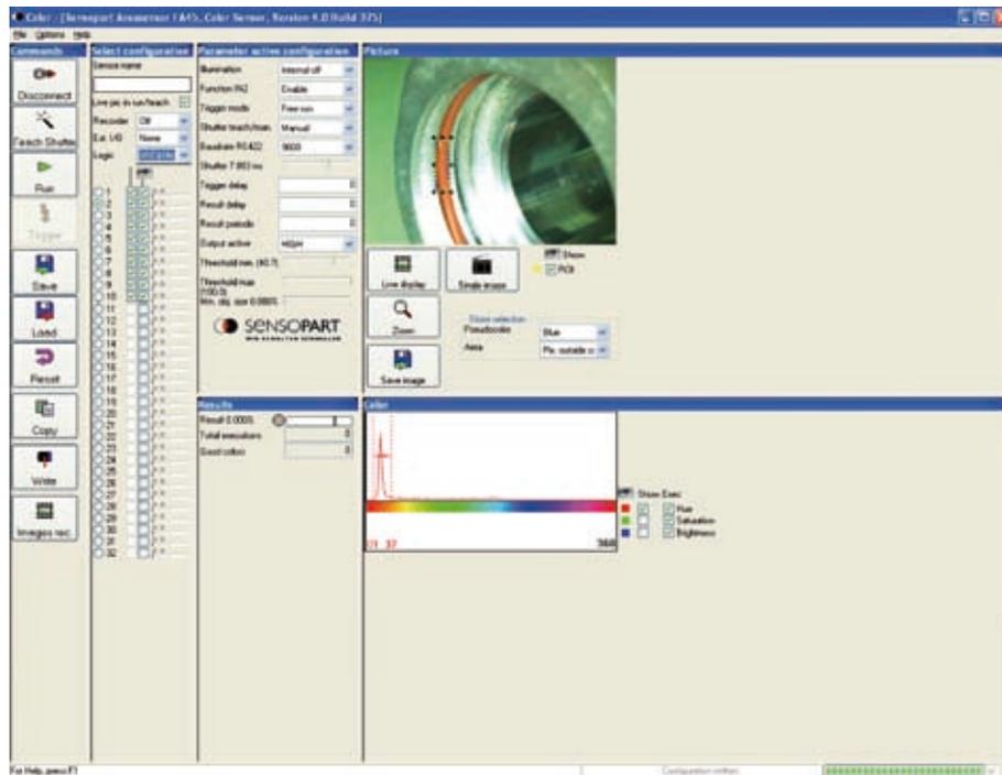
In an automated assembly process, the presence of a sealing ring (O-ring) in a cast part is to be checked.
