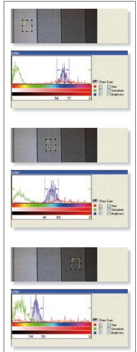
Evaluating coloured objects in the HSV colour model (colour value, saturation and brightness) achieves a high selectivity.
