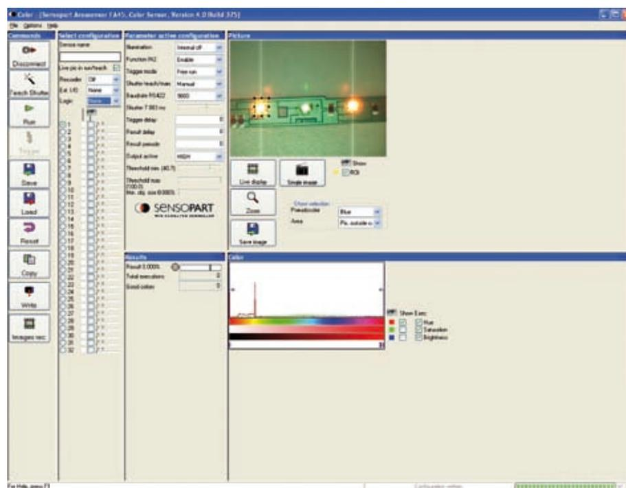
Colour shade can be used to determine whether a LED has been fitted in the right place in the right colour. Brightness determines whether a LED is on or not.
