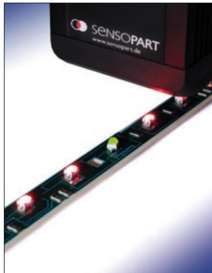
Detection of active, luminous objects such as LEDs or displays are no problem for the FA 45 colour sensor. It checks whether the LED is on and checks its colour.
