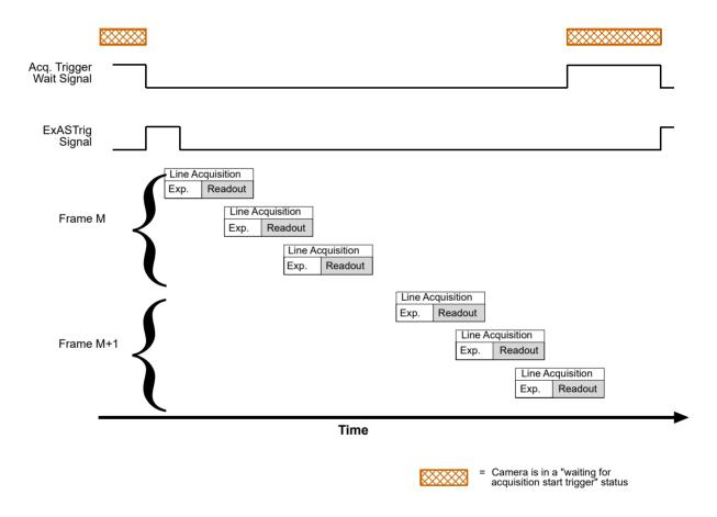
Fig. 47: Acquisition Trigger Wait Signal
