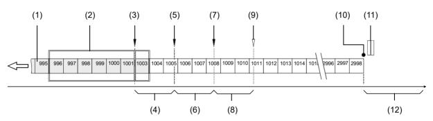
Fig. 12: Combination of Threshold Resend Mechanism and Timeout Resend Mechanism
