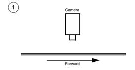
The conveyor is moving forward and the encoder is generating forward ticks. Whenever the module receives a forward tick, it outputs a trigger signal. The reverse counter is at 0.
