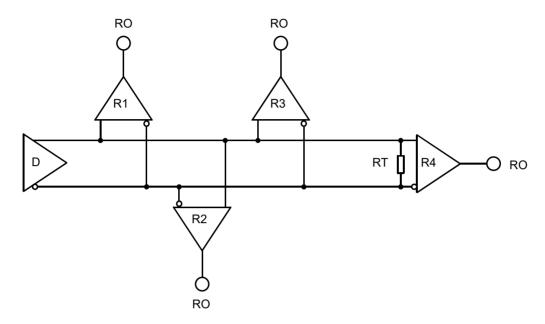
Fig. 20: RS-422 Interface Circuit Including Four Receivers as an Example
