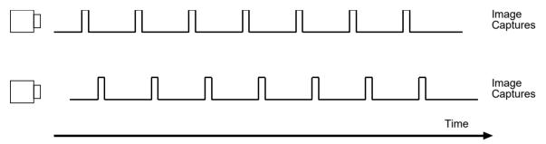
Fig. 63: Example A: Without PTP: Cameras Capturing at the Same Frame Rate, but Running Asynchronously
