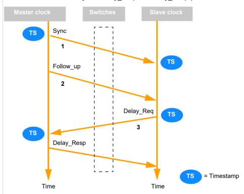
Fig. 61: PTP Clock Synchronization: Message Exchange Sequence
