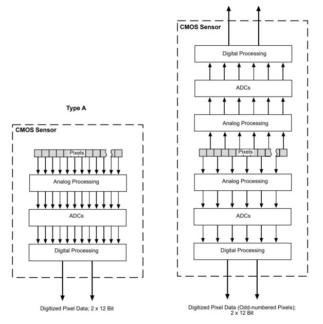
Fig. 14: CMOS Sensor Architecture. Type A is a 2k Sensor or 2k Sensor Segment with a Pixel Size of 7  $\mu$ m x 7  $\mu$ m and Type B is a 4k Sensor Segment with a Pixel Size of 3.5  $\mu$ m x 3.5  $\mu$ m.
