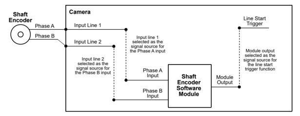
Fig. 51: Typical Shaft Encoder Module Implementation
