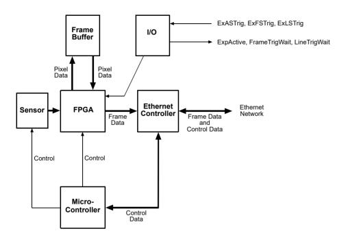
Fig. 15: Camera Block Diagram
