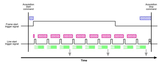
Fig. 34: Use Case 5 - Continuous Frame Mode with Acquisition Start Triggering Set to Off, Frame Start and Line Start Triggering Set to On, and TriggerPartialClosingFrame set to False
