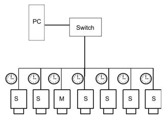
Possibility A: One camera has the master clock (M); the other cameras have slave clocks (S).
