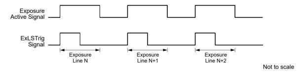
Fig. 46: Exposure Active Signal
