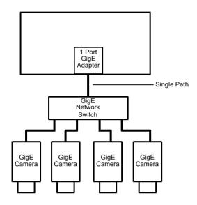
Fig. 13: Multiple Cameras on a Network
