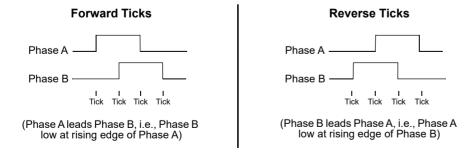
Fig. 52: Software Module Direction Sensing
