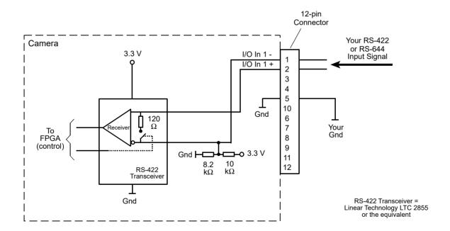
Fig. 19: Inputting RS-422 or RS-644 Signals
