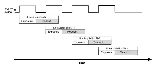
Fig. 40: Overlapped Exposure and Readout
