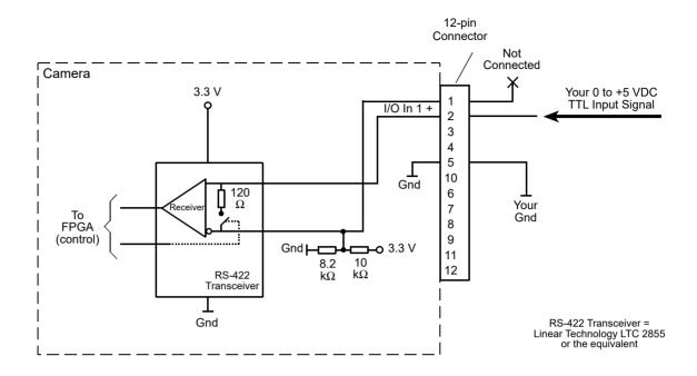
Fig. 21: Inputting Low Voltage TTL Signals
