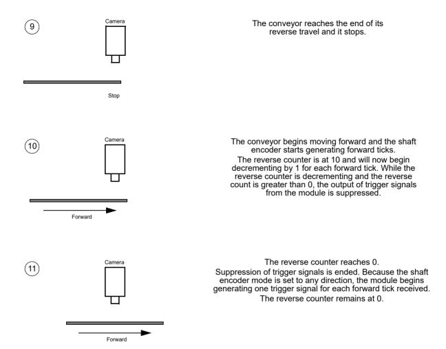
There are two main things to notice about this example. First, because the encoder mode is set to any direction, ticks from the shaft encoder will cause the module to output trigger signals regardless of the conveyor direction, as long as the reverse counter is not incrementing or decrementing. Second, the reverse counter will compensate for conveyor jitter regardless of the conveyor direction.
