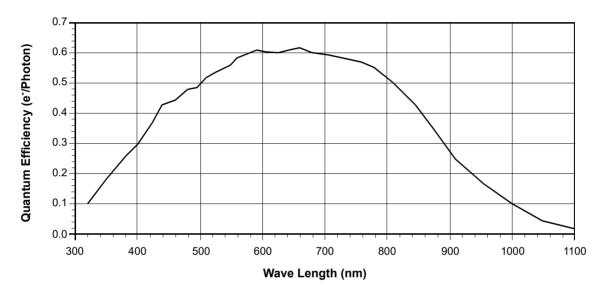
Fig. 2: Quantum Efficiency of the Monochrome Sensor in 12 Bit Depth Mode (Based on Sensor Vendor Information)
