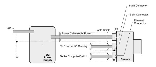
Fig. 17: Grounding Scheme for Power Supply, Power Cable, and Camera
