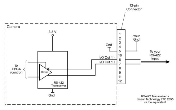
Fig. 22: RS-422 Output Signal
