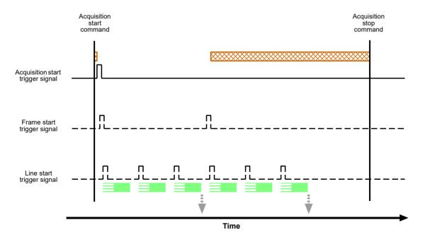
Fig. 37: Use Case 8 - Continuous Frame Mode with Acquisition Start Triggering Set to On and Frame Start and Line Start Triggering Set to Off
