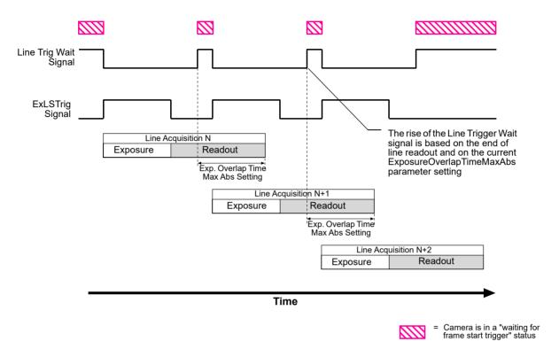
Fig. 50: Line Trigger Wait Signal with the Trigger Width Exposure Mode
