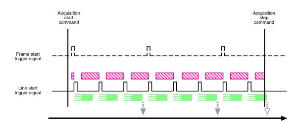
Fig. 36: Use Case 7 - Continuous Frame Mode with Acquisition Start and Frame Start Triggering Set to Off and Line Start Triggering Set to On
