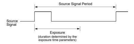
Fig. 29: Timed Exposure with RisingEdge Line Start Triggering
