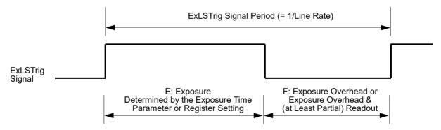
Fig. 45: Relation of the ExLSTrig Signal Period and Periods E and F for Regular Line Acquisition in Trigger Width Exposure Mode
