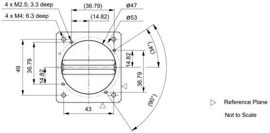
Fig. 3: Mechanical Dimensions (in mm)
