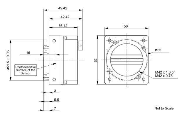
Fig. 7: M42 x 1.0 or M42 x 0.75 FBD 16 mm Mount Adapter on a racer GigE Camera; Dimensions in mm
