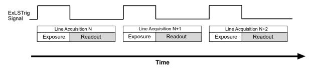
Fig. 39: Non-overlapped Exposure and Readout
