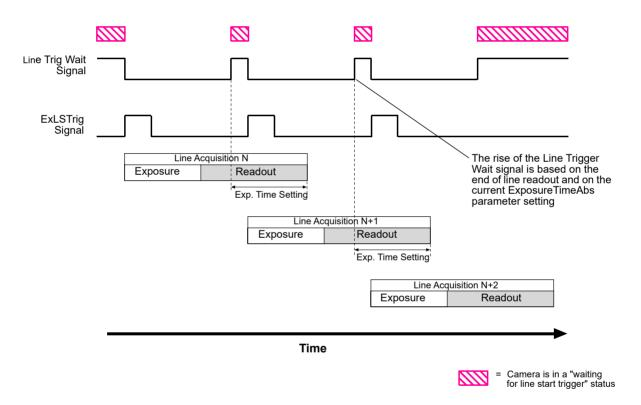
Fig. 49: Line Trigger Wait Signal with the Timed Exposure Mode
