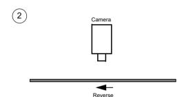
The conveyor jitters and moves briefly in reverse. During this reverse movement, the shaft encoder generates 5 reverse ticks.
