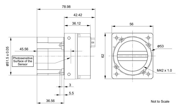
Fig. 8: M42 x 1.0 FBD 45.56 mm Mount Adapter on a racer GigE Camera; Dimensions in mm
