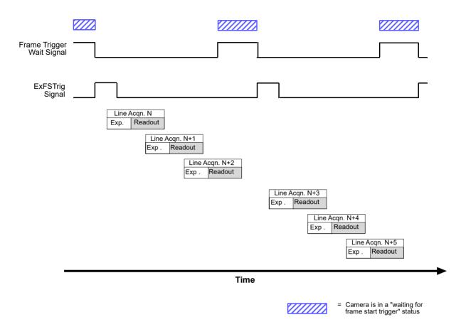
Fig. 48: Frame Trigger Wait Signal
