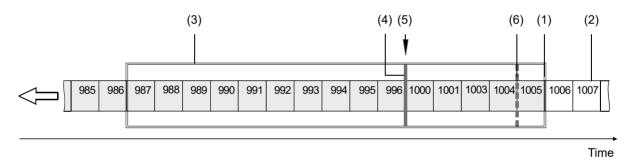
Fig. 10: Example of a Receive Window with Resend Request Threshold & Resend Request Batching Threshold
