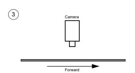
The conveyor resumes forward motion and the shaft encoder module begins generating forward ticks. The reverse counter will decrement by 1 for each forward tick. While the reverse counter is decrementing, the output of trigger signals from the module is suppressed.
