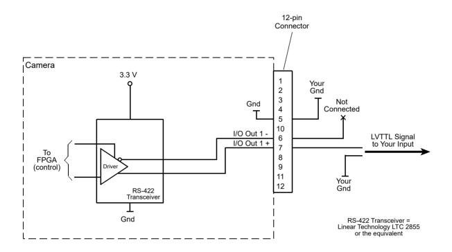
Fig. 24: Output Line Wired for Use with an LVTTL Input
