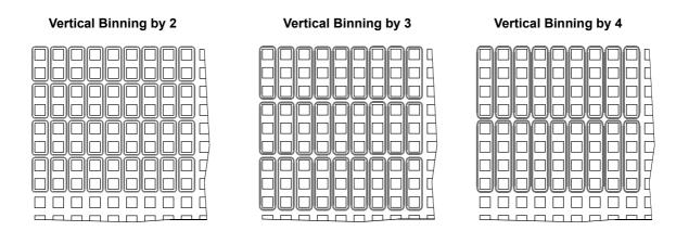
Fig. 72: Vertical Binning
