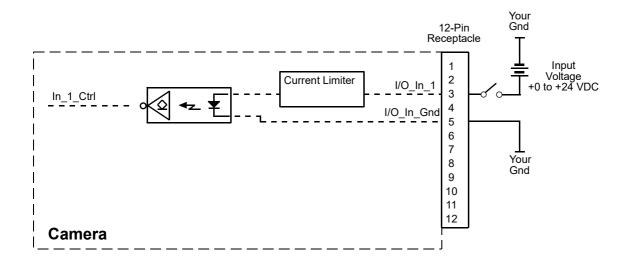
Fig. 30: Typical Voltage Input Circuit
