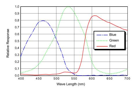
Fig. 7: scA640-70gc Spectral Response
