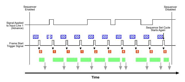
Fig. 68: Sequencer in Controlled Sequence Advance Mode with Line 1 as the Sequence Control Source
