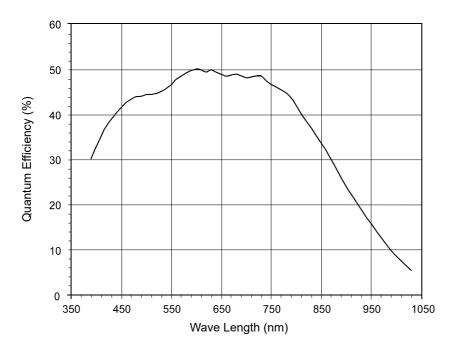
Fig. 2: scA750-60gm Spectral Response
