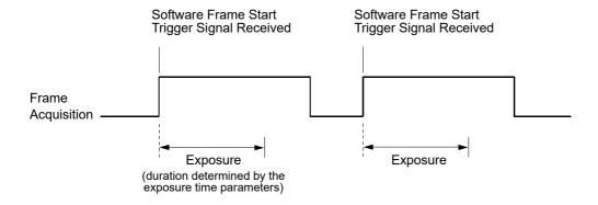
Fig. 38: Frame Acquisition with a Software Frame Start Trigger
