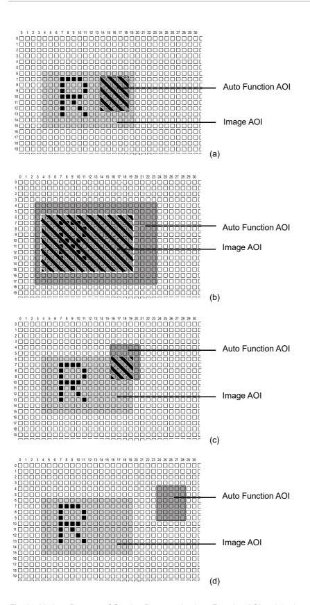
Fig. 81: Various Degrees of Overlap Between the Auto Function AOI and the Image AOI
