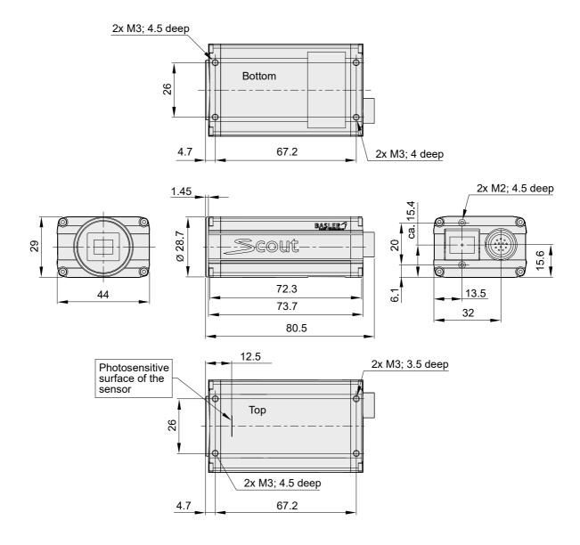
Fig. 14: Mechanical Dimensions (in mm) for Cameras with an Optional CS-mount Lens Adapter
