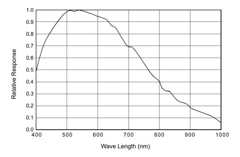
Fig. 5: scA1400-17gm and scA1400-30gm Spectral Response
