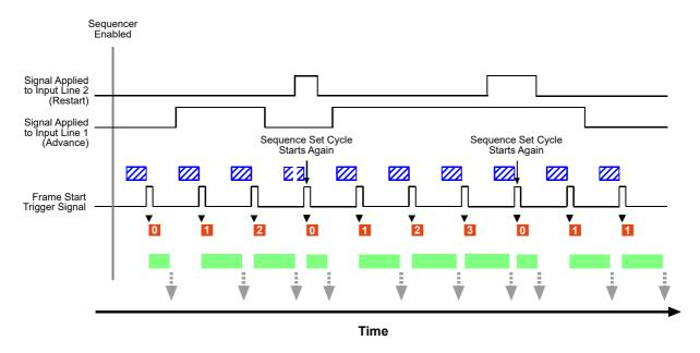
Fig. 69: Sequencer in Controlled Sequence Advance Mode with Line 1 as the Sequence Control Source and Synchronous Restart Controlled by Line 2
