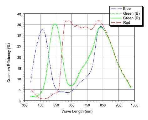
Fig. 8: scA750-60gc Spectral Response
