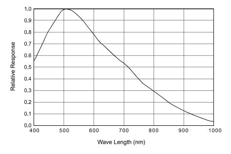
Fig. 3: scA1000-30gm Spectral Response
