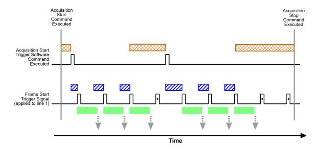
Fig. 50: Use Case 4 - Acquisition Start Trigger On and Frame Start Trigger On
