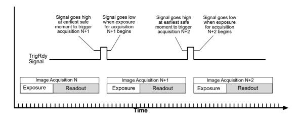
Fig. 56: Trigger Ready Signal
