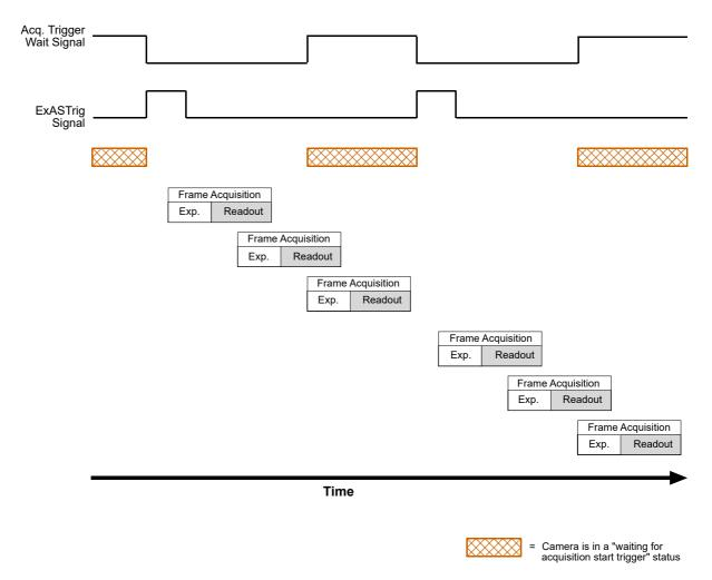
Fig. 57: Acquisition Trigger Wait Signal
