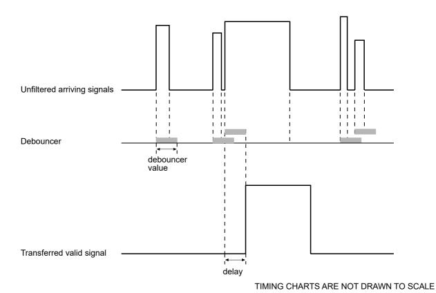
Fig. 82: Filtering of Input Signals by the Debouncer
