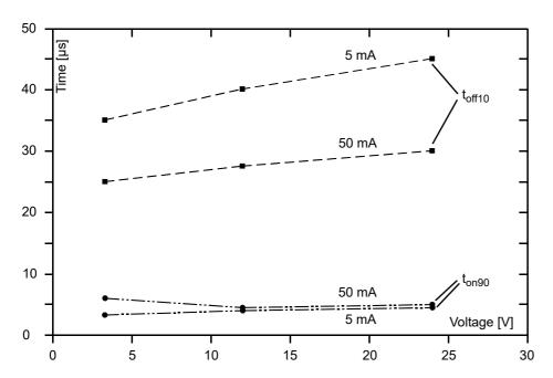
Fig. 33: Dependence of  $t_{on90}$  and  $t_{off10}$  on Voltage, for Different Load Currents; Measured for an Individual Camera as an Example
