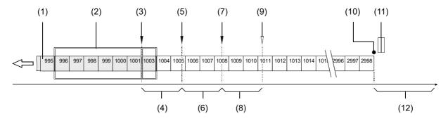
Fig. 22: Combination of Threshold Resend Mechanism and Timeout Resend Mechanism
