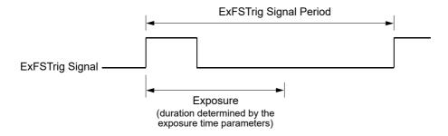
Fig. 39: Timed Exposure with Rising Edge Triggering
