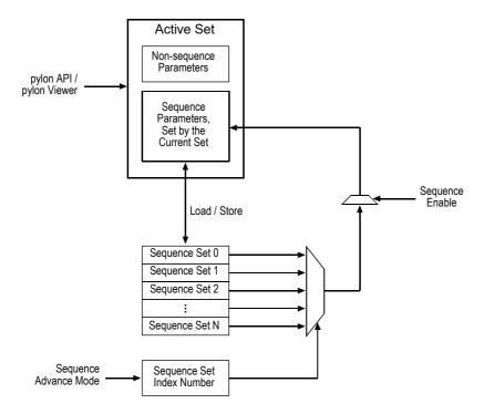
Fig. 64: Sequence Feature Block Diagram
