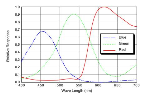
Fig. 10: scA1300-32gc Spectral Response
