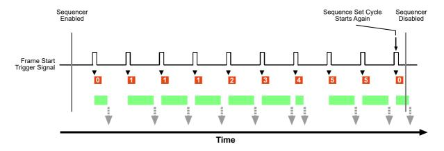
Fig. 65: Sequencer in Auto Sequence Advance Mode
