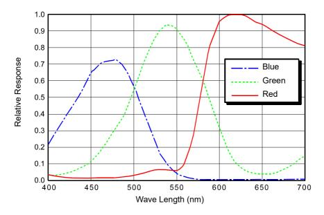
Fig. 11: scA1400-17gc and scA1400-30gc Spectral Response
