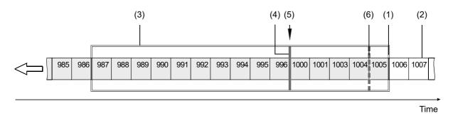
Fig. 20: Example of a Receive Window with Resend Request Threshold & Resend Request Batching Threshold
