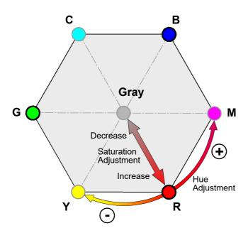
Fig. 61: Hue and Saturation Adjustment In the Color Hexagon. Adjustments Are Indicated for Red as an Example
