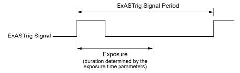
Fig. 43: Timed Exposure with Rising Edge Triggering
