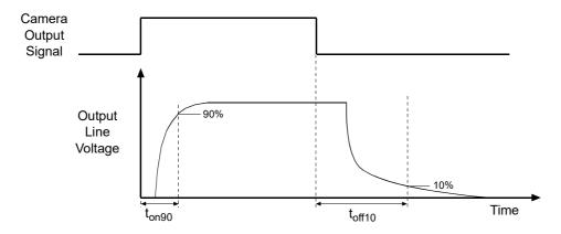
Fig. 32: Output Line Response Times
