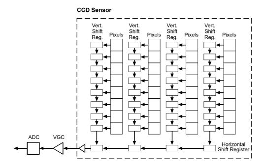
Fig. 24: CCD Sensor Architecture
