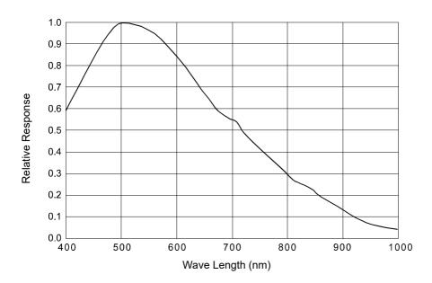
Fig. 1: scA640-70gm Spectral Response Spectral Response
