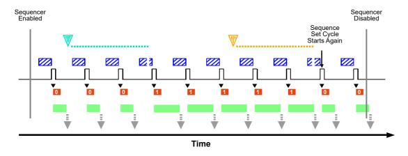
Fig. 70: Sequencer in Controlled Sequence Advance Mode with Disabled as the Sequence Control Source and Asynchronous Advance and Restart
