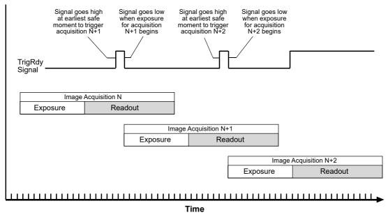
Fig. 55: Trigger Ready Signal
