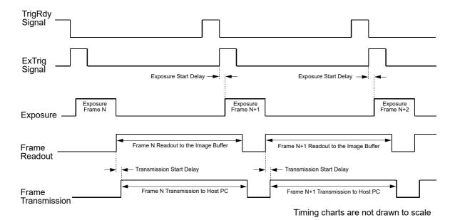
Fig. 58: Exposure Start Controlled with an ExTrig Signal
