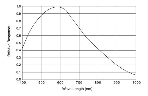
Fig. 4: scA1300-32 gm Spectral Response
