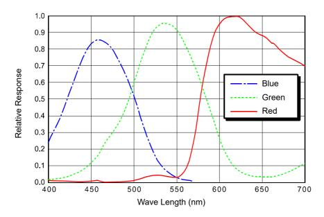
Fig. 12: scA1600-14gc and scA1600-28gc Spectral Response
