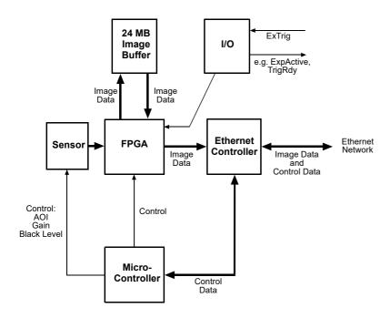
Fig. 27: Camera Block Diagram
