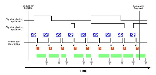
Fig. 71: Sequencer in Free Selection Mode
