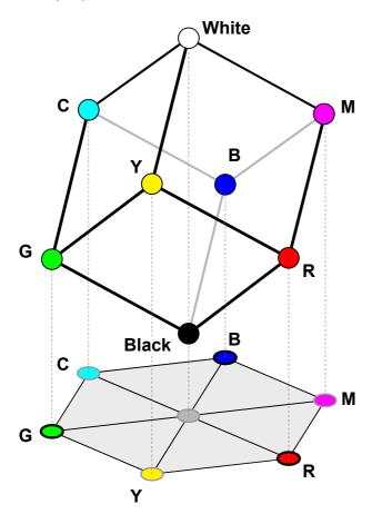
Fig. 60: RGB Color Cube With YCM Secondary Colors, Black, and White, Projected On a Plane
