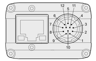
Fig. 29: Pin Numbering for the 12-pin Receptacle
