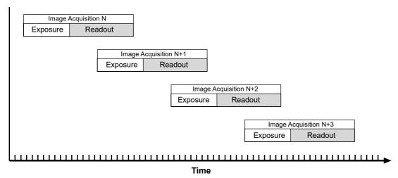
Fig. 52: Overlapped Exposure
