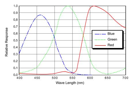
Fig. 9: scA1000-30gc Spectral Response
