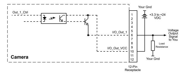
Fig. 31: Typical Voltage Output Circuit
