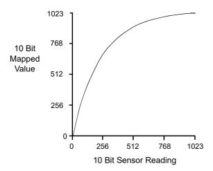
Fig. 79: Lookup Table with Values Mapped for Higher Camera Output at Low Sensor Readings
