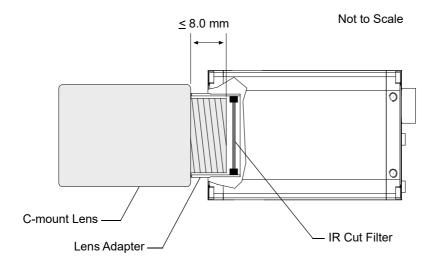
Fig. 19: Maximum Lens Thread Length on Color Cameras
