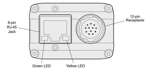
Fig. 28: Camera Connectors and LED
