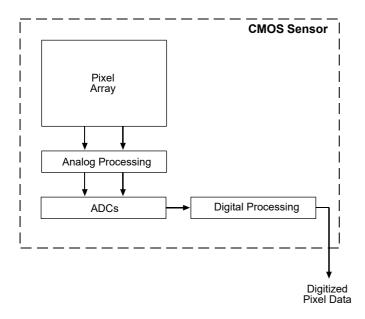
Fig. 26: CMOS Sensor Architecture
