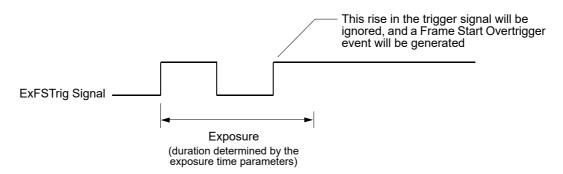
Fig. 40: Overtriggering with Timed Exposure
