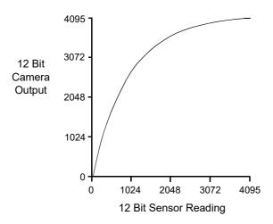
Fig. 77: Lookup Table with Values Mapped for Higher Camera Output at Low Sensor Readings
