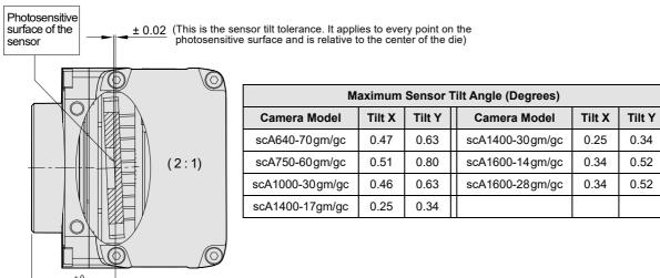
Fig. 18: Sensor Positioning Accuracy for Cameras (90° Head) with the Standard C-mount Lens Adapter (in mm unless otherwise noted)
