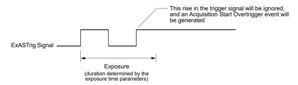
Fig. 44: Overtriggering with Timed Exposure
