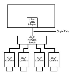
Fig. 23: Multiple Cameras on a Network
