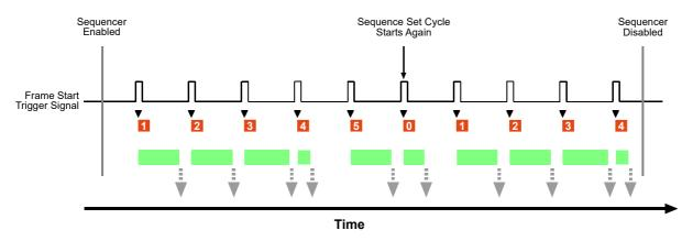
Fig. 66: Sequencer in Controlled Sequence Advance Mode with Always Active as the Sequence Control Source
