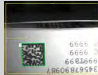
Printed codes on pharmaceutical packaging Simultaneous searching for ECC200 or barcodes (e.g. EAN 13) is possible. Besides reading the code, the presence of plain text can be checked via object detection.
