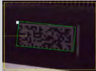
Code with low contrast Becomes readable through high tolerance, even compared to low-contrast codes.
