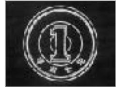
Sample Edge Detection Using a 1-Yen Coin
