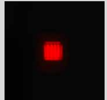
(Fig. top) Easy alignment: F 55 sensors can be easily set up by just one person thanks to the bright light spot which is clearly visible even in broad daylight. This is even valid for the through beam sensor as teach-in can be carried out either on the transmitter or receiver.
