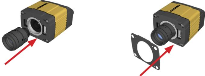
**3** Attach the reader to the bracket subassembly using four M3x10 mm flat head cap screws.
