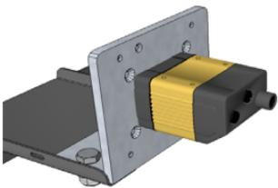
4 Attach the M3x25 mm flat head cap screw to the FOVE-bracket using an M3 hex nut.
