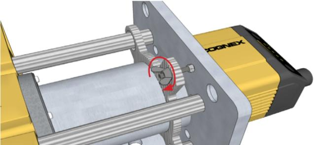
For attaching a DataMan 503 reader to Xpand 15, follow the steps highlighted below.
