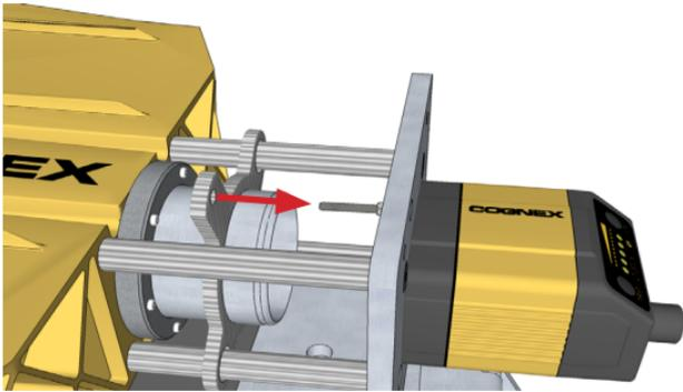
**i** A small amount of extra force might be needed to have the lens cover snap into place properly against the o-ring in the FOVE-bracket.
