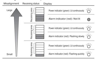
[Countermeasure]: Move the light axis to the bottom side.
