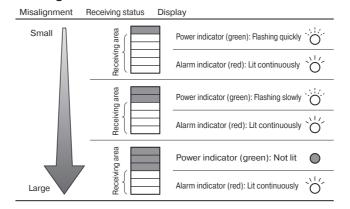
[Countermeasure]: Move the light axis to the top side.
