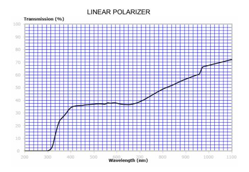
All Smart Vision Lights have a linear Polarizer available. Polarizing filters can reduce reflections on specular surfaces. A polarizer can be added in the field by using push in clips. Lights can also be ordered with polarizer internally installed.
