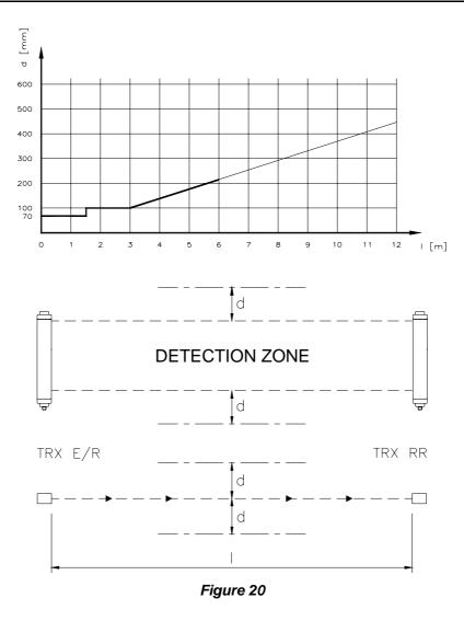
After installing the system, check whether any reflecting surfaces intercept the beams, first in the centre and then in the vicinity of the active unit.
