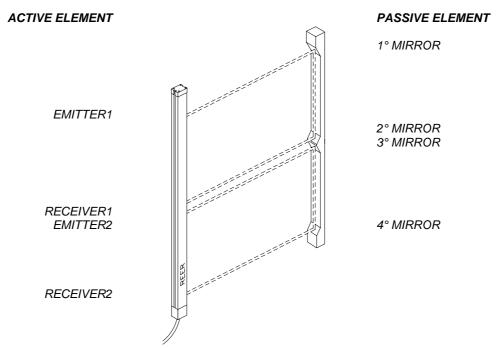
Figure 2 - MI TRX / J TRX with 3 beams
