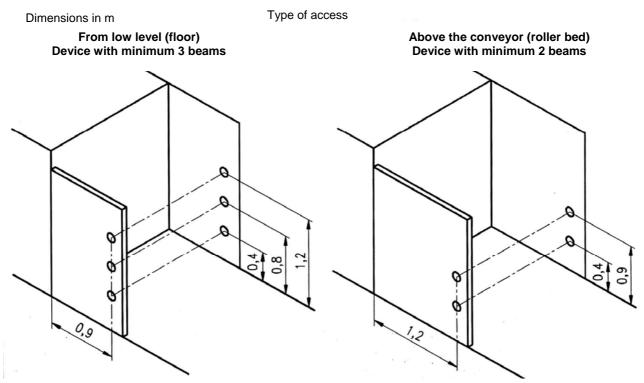
Figure 17: Protection of the opening with MI/ML/MT TRX light curtain and mechanical side guards.
