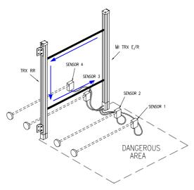
Figure 7 - Connection with 4 external sensors
