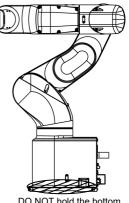
DO NOT hold the bottom of the base by hand.
