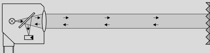
With retroreflective photoelectric sensors one speaks of the autocollimation principle when the light reflected from the reflector travels parallel to itself (i.e. within itself). The light emitted by the sensor hits a reflector and is reflected. The reflected light is then deflected to a receiver by a semi-transparent mirror and evaluated.
