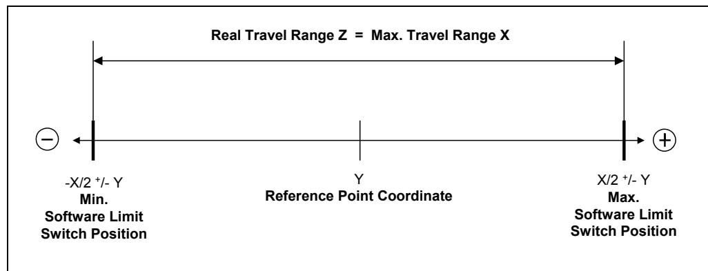
Figure 16: Software limit switch positions / Reference point coordinate
