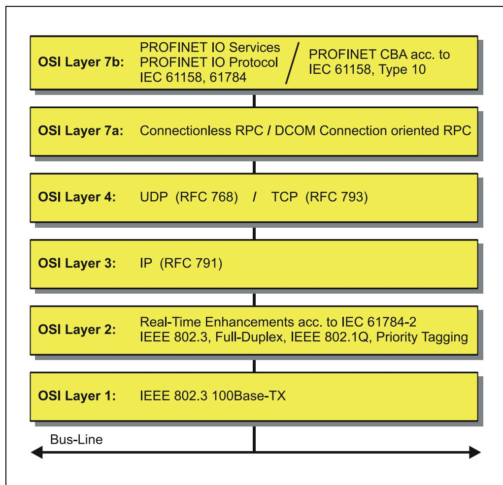
Figure 1: PROFINET organized in the ISO/OSI layer model
