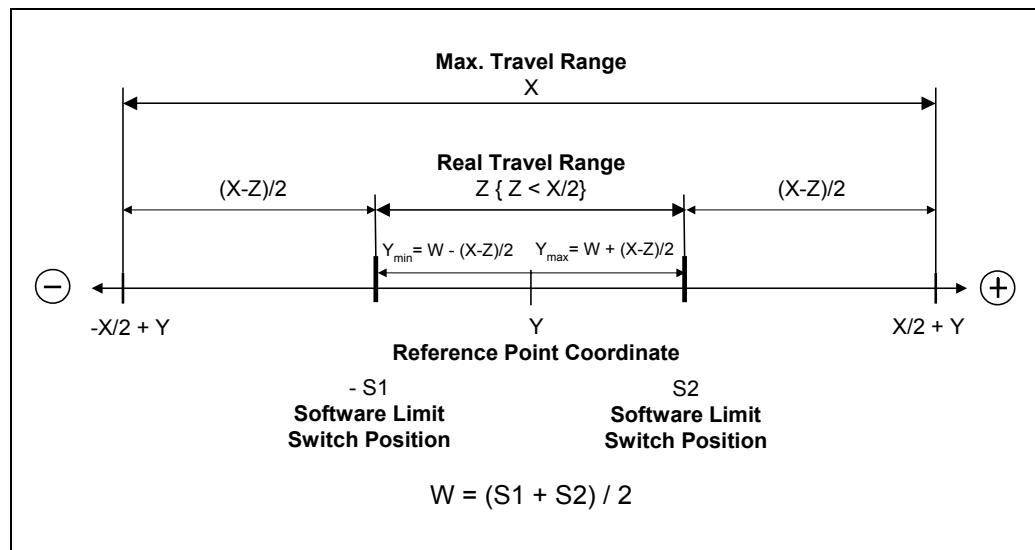
Figure 17: Max. Reference point coordinate,  $Z < X/2$
