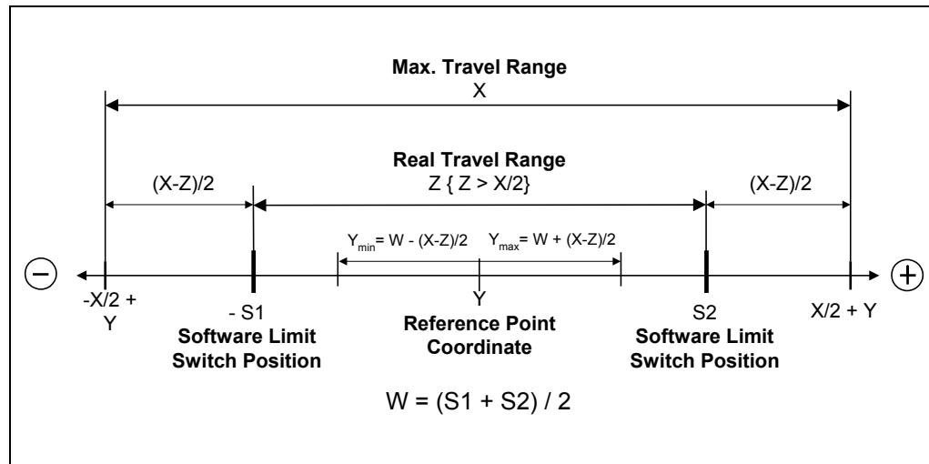
Figure 18: Max. Reference point coordinate,  $Z > X/2$
