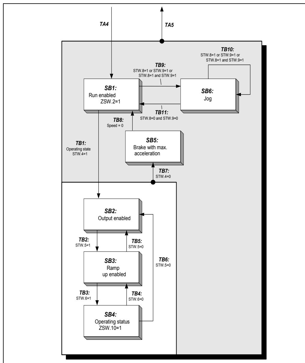
Figure 11: PROFIDrive state machine, speed control mode
