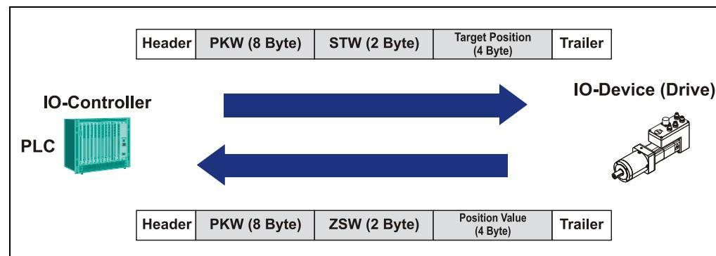
Figure 6: Cyclic communication with PKW channel
