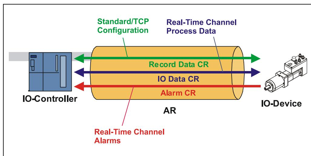
Figure 22: Device communication
