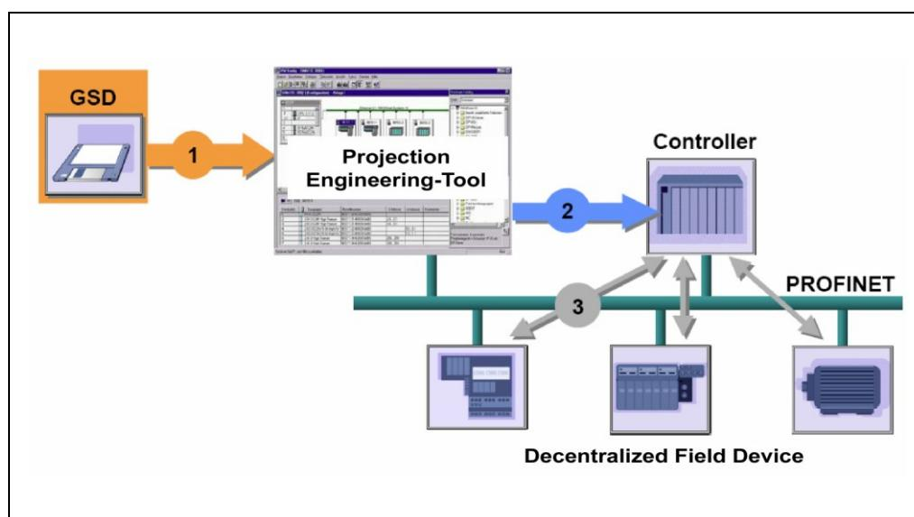
Figure 21: GSDML file for the configuration [Source: PROFIBUS International]
