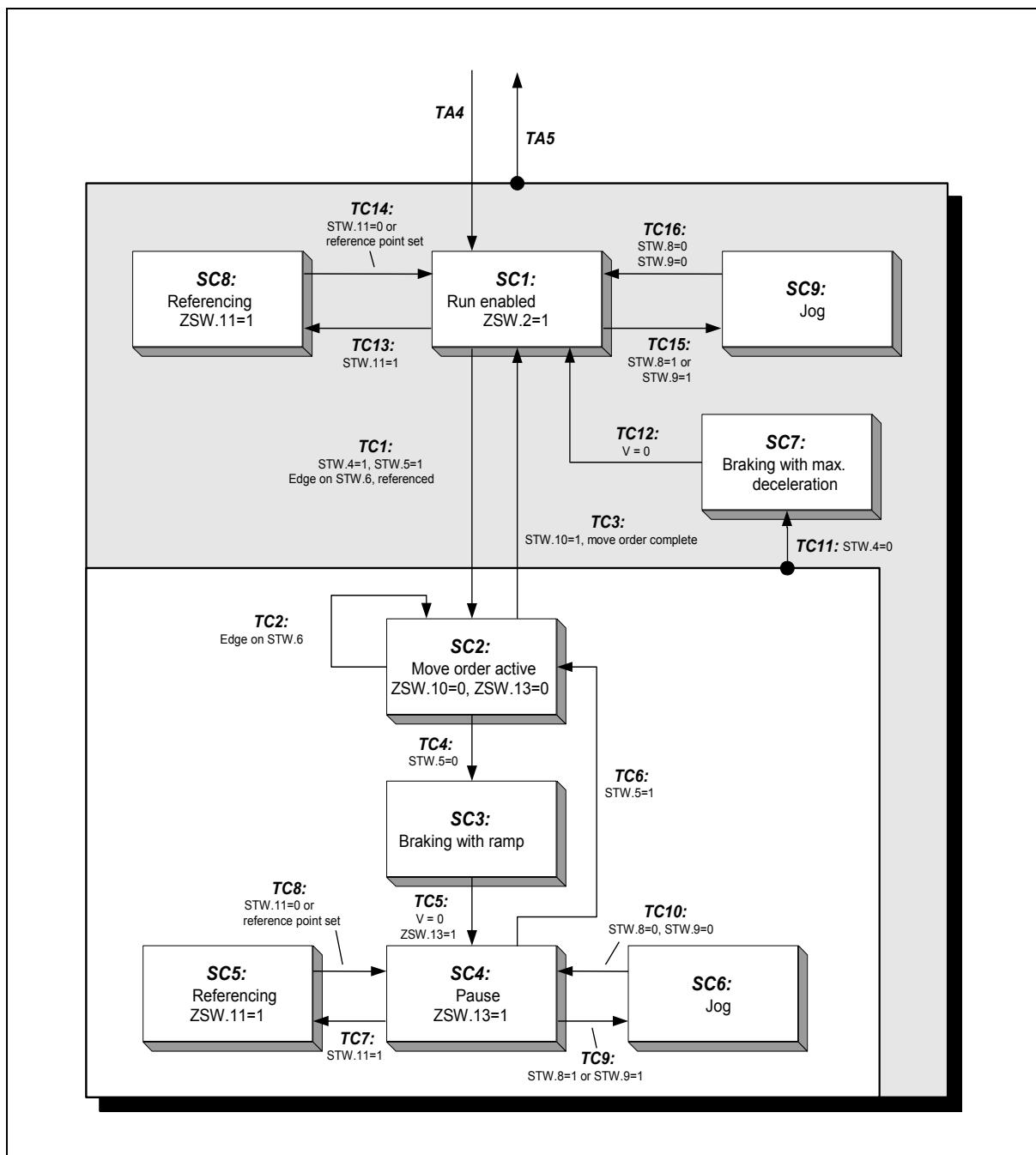
Figure 9: PROFIdrive state machine, positioning mode
