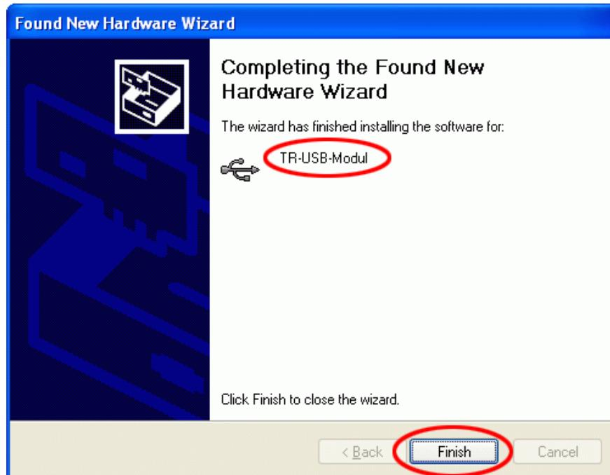
After this the *Found New Hardware Wizard* is started again for the **Serial Port**. The proceeding is the same as before. After finishing of the installation the PC adapter is functional.
