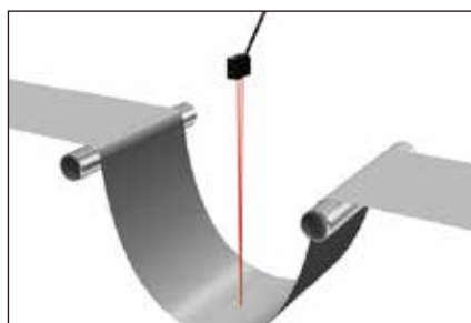
Loop control for sheet materials
