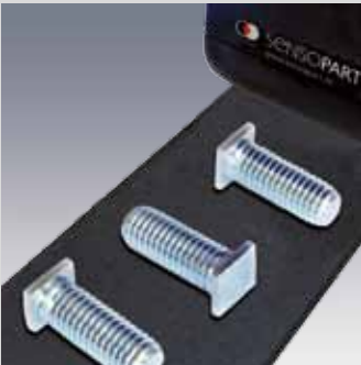
Position and position tolerance measurement: The sensor "learns" the contours and their direction from a picture, and reacts reliably to deviations. The sensor responds correctly even if a nut is the wrong way round.
