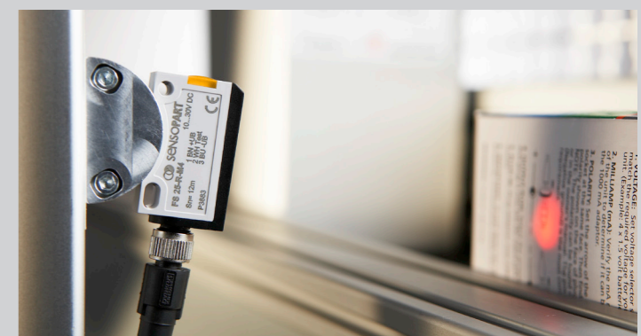
Object detection: Whether in handling or in assembly, whether large or small objects made of paper or metal – FT 25-RHD and FT 25-RLH photoelectric proximity sensors with background suppression reliably detect the most varied of objects – even with interfering backgrounds.
