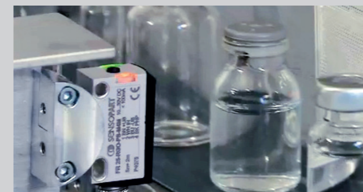
Detection of transparent objects: The FR 25-RGO photoelectric proximity sensor has been especially designed for detecting transparent objects. It offers absolutely precise and reproducible switching behaviour thanks to its autocollimation principle and automatic adaptation of the switching threshold (the DELTA function).
