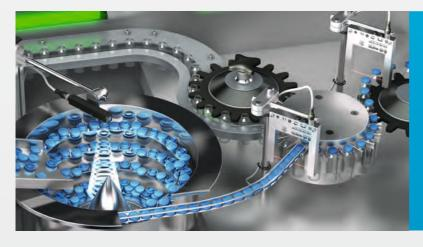
Feed control and fast trigger sensor in a sealing machine
