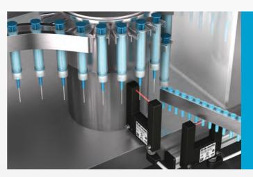
Accumulation monitoring OGU 081 G3-T3 The "Power" sensor mode reduces cleaning cycles
