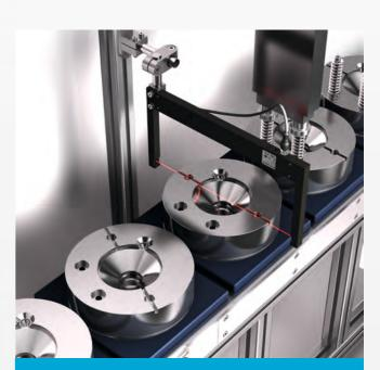
Position monitoring of the groove in the circular piece
