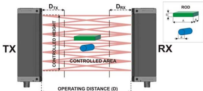
The beam interruption due to the passage of an object inside the controlled area causes the closing of the switching output and the variation of the device analogue output signal. Small objects can be detected (reaching dimensions of only 0.5 mm) and with a reduced surface area.
