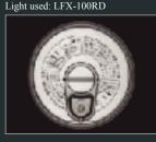
With the LFX at distance of 295 mm from the light to the object, the more collimated light shows the smaller ridges in the can surface clearly. Light used: LFX-100RD
