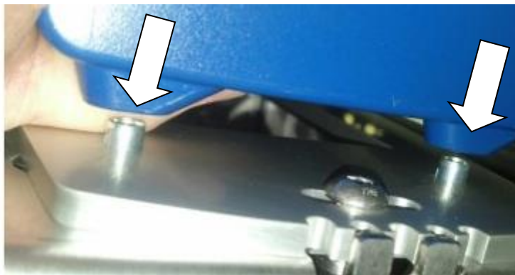
Figure 70: Placing DM3610 on the hollow Spirol™ spring dowel
