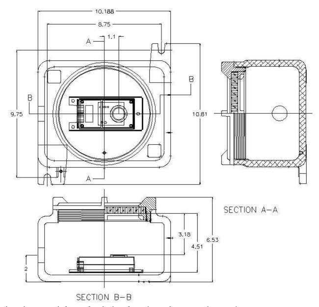
Enclosure is constructed of copper free aluminum for maximum salt water corrosion protection. Fasteners (M4x8 BHSCS) to mount the DVT Legend 500 series SmartImage Sensor are included. Camera can be raised inside the enclosure by 38mm to better accommodate wide angle lenses. Enclosure meets NEMA 4 standards. Enclosure is tapped for 1" NPT conduit.
