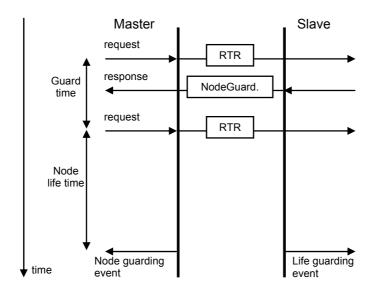
**100C-00 Guard time**: interval between two RTR messages. **Node life time**: maximum time available for the encoder to
