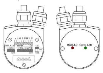
The connection cap is fitted with two PG9 cable glands for bus-IN, bus-OUT and supply voltage connections. The bus cables can be connected directly to the terminal connectors in front of each cable gland. It is recommended to use CANbus certificated cables.
