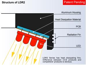
With conventional construction, LED lights are not able to dissipate heat with total efficiency due to the gap between the PCB and aluminum housing.
