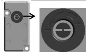
The emitter is equipped with a trimmer which let user change the emission power. The operating distance increases rotating the trimmer clockwise. The emission power reduction it is useful to decrease passive reflections when the maximum operating distance it is not required. Trimmer rotation is limited to 260°. Do not apply a torque greater than 35 Nmm.
